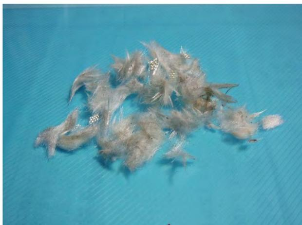
Fig.8 Recovered glass fiber from epoxy board by using tar prepared at 300°C
