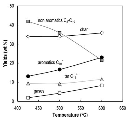
Fig. 1. Effect of temperature on the yield of the different lumps in the 425-600 °C range.
